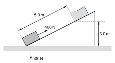
Part of the work done increases the gravitational potential energy E of the crate and the rest is work done W against friction.
