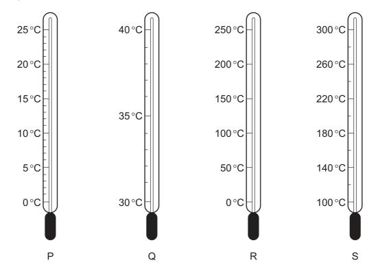
Which thermometer has the greatest sensitivity and which thermometer has the greatest range?
